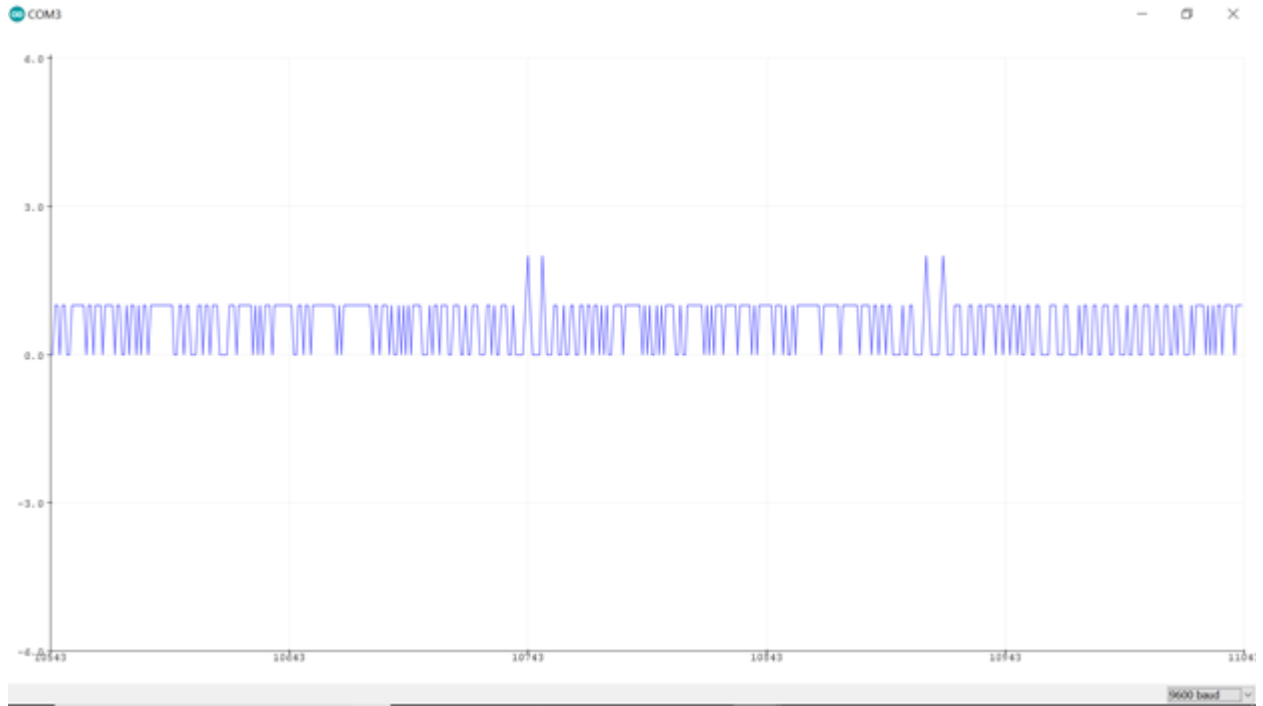
Graph (11) - |a| vs. time approximation for bending over, sitting down (from standing), standing up (from sitting), and walking on a flat surface.
